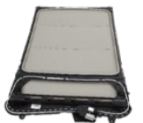
ELECTRICAL ROOF SUNSHADE
